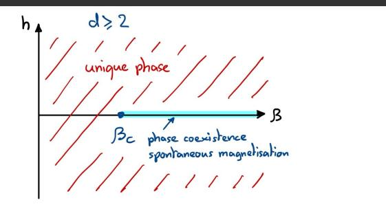
FIGURE 1.1. Phase diagram of the **Ising model**, and of the **XXZ** model for  $J^{(3)} > J^{(1)} = J^{(2)} \ge 0$ , for all dimensions  $d \ge 2$ .
